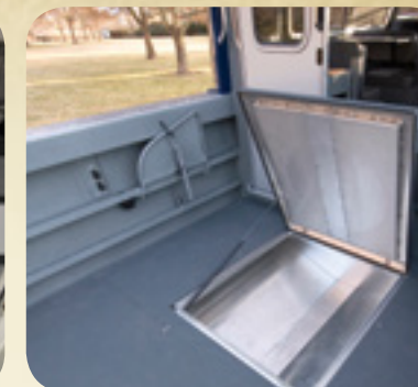
Oversized, fully insulated, sub-floor fish box. Extra-oversized fish box available on 28' and 30' models.
