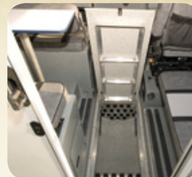
Optional sub-floor, high security, intelligent storage for up to 12 rods. Additional rod storage in side trays and overhead rocket launchers.
